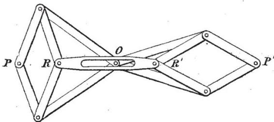
at O; and the poles R and R' are connected together by a bar with a slot in it, through which the pin which forms the pivot at O passes. Then if P, R, P', R', are constrained to keep in a straight line, P and P' can approach or recede from O, only in such a way that, if there is a lens of proper focal length at O, P and P' will always be conjugate foci.
