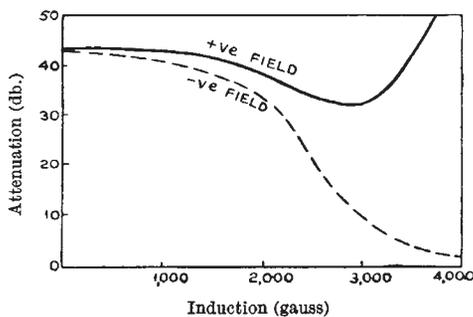
Fig. 1. Specimens of ferroxcube B2 at 10,200 Mc./s., with the following diameters: 0.125 in. (upper graph); 0.562 in. (lower graph)
