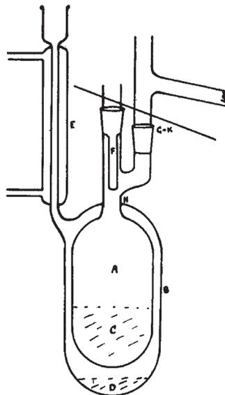
Fig. 1. *A*, internal flask, round or elongated, with all-glass sea at *H*; *B*, outer jacket; *C*, liquid for distillation; *D*, higher boiling point; *E*, water-jacketed condenser; *F*, thermometer pocket; *G*, ground joints; *H*, all-glass seal
