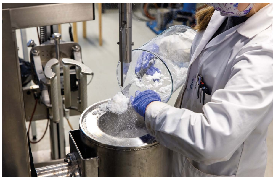
Recycling cellulose involves producing a pulp that can then be used to make new fibres.
