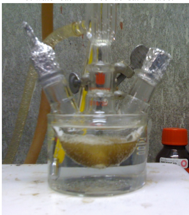
The setup with the round-bottom flask in A hot water bath with condensation tube.
