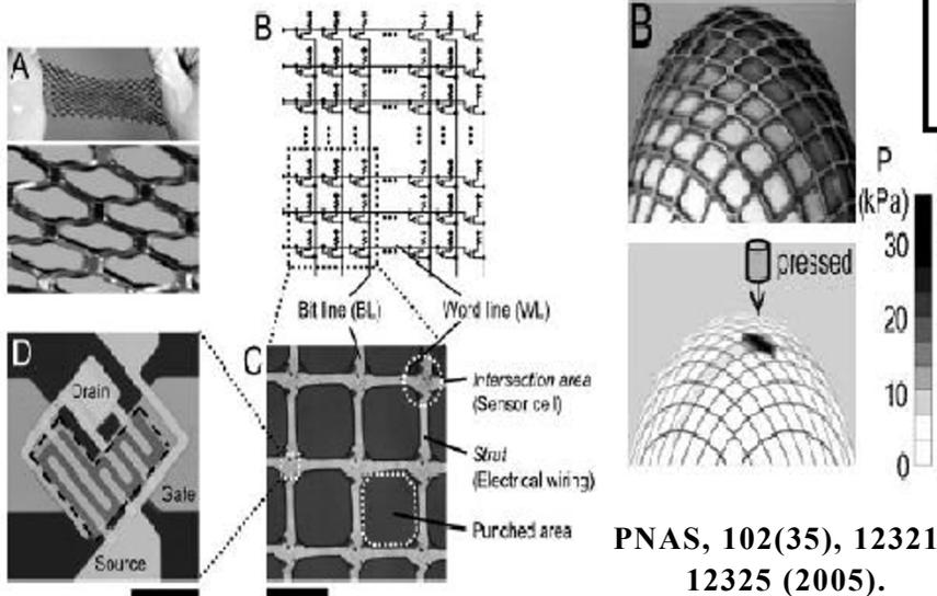
Conformal network of pressure sensors
