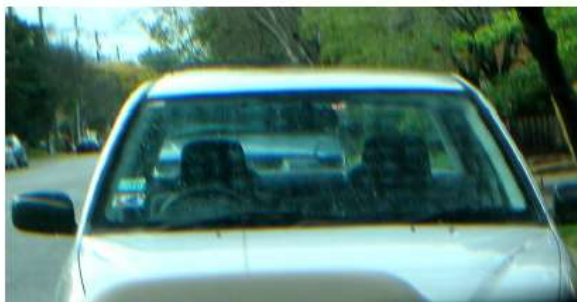
Polarizing sunglasses reveal stress in car window (see text for explanation.)
