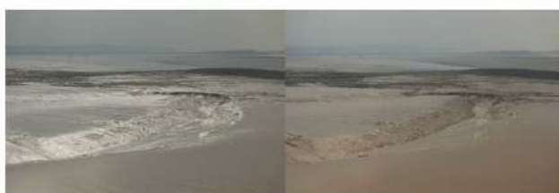
Effect of a polarizer on reflection from mud flats. In the picture on the left, the polarizer is rotated to transmit the reflections as well as possible; by rotating the polarizer by 90^\circ (picture on the right) almost all specularly reflected sunlight is blocked.
