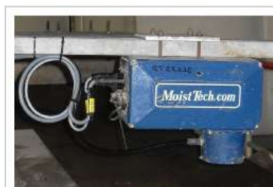
NIR sensor for moisture measurement installed on a belt conveyor
