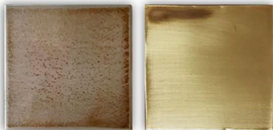
**Fig. 10** Macro-photos of PHS/PEOX +  $\text{CaCl}_2$  on steel (left) and on brass (right) after 48 h of drying. Corrosion is observed to be higher in the areas where more coating accumulated after application
