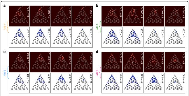
**Fig. 4 Nonlinear dynamics in fractal array with** r = 0.5a. Rich nonlinear dynamics and gradual transition to the localization at the highest power levels as observed for the excitations of sites 1-4 in  $G_3$  fractal array. The arrangement of panels is the same as in Fig. 3. Arrows in experimental panels indicate position of the input excitation
