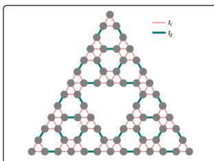
Fig. 7 Schematic illustration of third generation  $G_3$  of the Sierpiński gasket. The intra-cell couplings between sites (gray circles) are indicated in this plot with thin red lines, while inter-cell couplings are indicated with thick blue lines. The intra-cell and inter-cell coupling strengths are given by  $t_1$  and  $t_2$ , respectively
