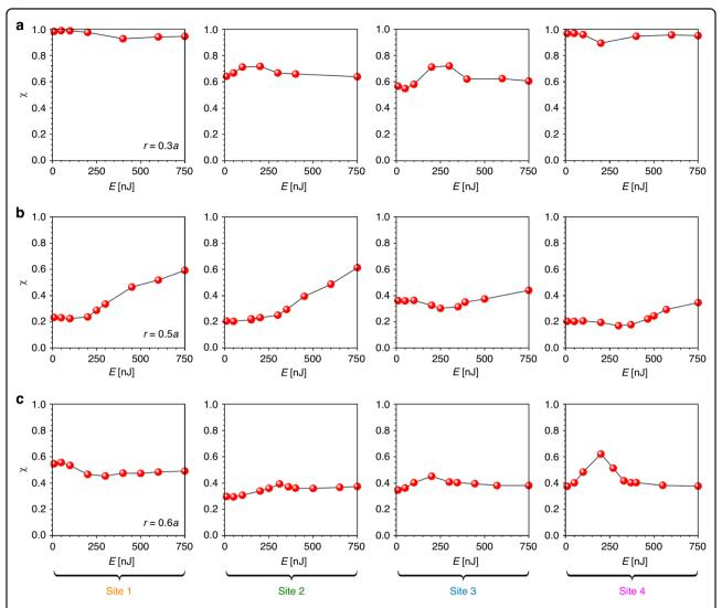
**Fig. 6 Experimentally measured output form-factor**. The form-factor as a function of pulse energy in case-2 arrays with r = 0.3a (**a**), r = 0.5a (**b**), and r = 0.6a (**c**). First to fourth columns correspond to excitations of sites 1 to 4, respectively. Standard deviation of measured form-factor does not exceed the size of red dots
