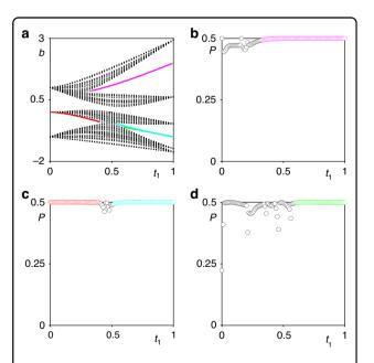
**Fig. 8 Real-space polarization index. a** Spectrum of the  $G_4$  fractal lattice versus intra-cell coupling strength  $t_1$  obtained from tight-binding model.  $\mathbf{b-d}$ ) Real-space polarization index corresponding to the corner state indicated by magenta color, red and cyan colors, and green color in  $(\mathbf{a})$
