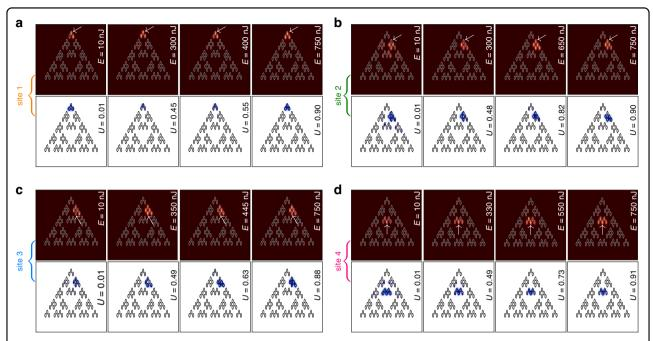
**Fig. 5 Observation of nonlinear states in fractal array with** r = 0.6a. Formation of the localized thresholdless nonlinear states for the excitation of sites 1 (**a**) and 4 (**d**) and rich nonlinear dynamics with the light switching between several closely located waveguides for excitation of sites 2 (**b**) and 3 (**c**) observed in  $G_3$  fractal array. Arrows in the experimental panels indicate position of the input excitation
