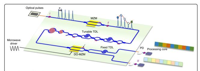
**Fig. 1 Schematic of the silicon photonic chip hosting the analog parallel processor (APP).** The optical pulses generated by a comb source perform temporal discretization of the broadband RF signal driving the Mach-Zehnder modulator (MZM). A tunable time delay line (TDL) synchronizes the discretized signal with the microwave driver of the dual-output modulator (DO-MZM) used as a switch to parallelize the temporal discrete signal into the two output channels<sup>12</sup>
