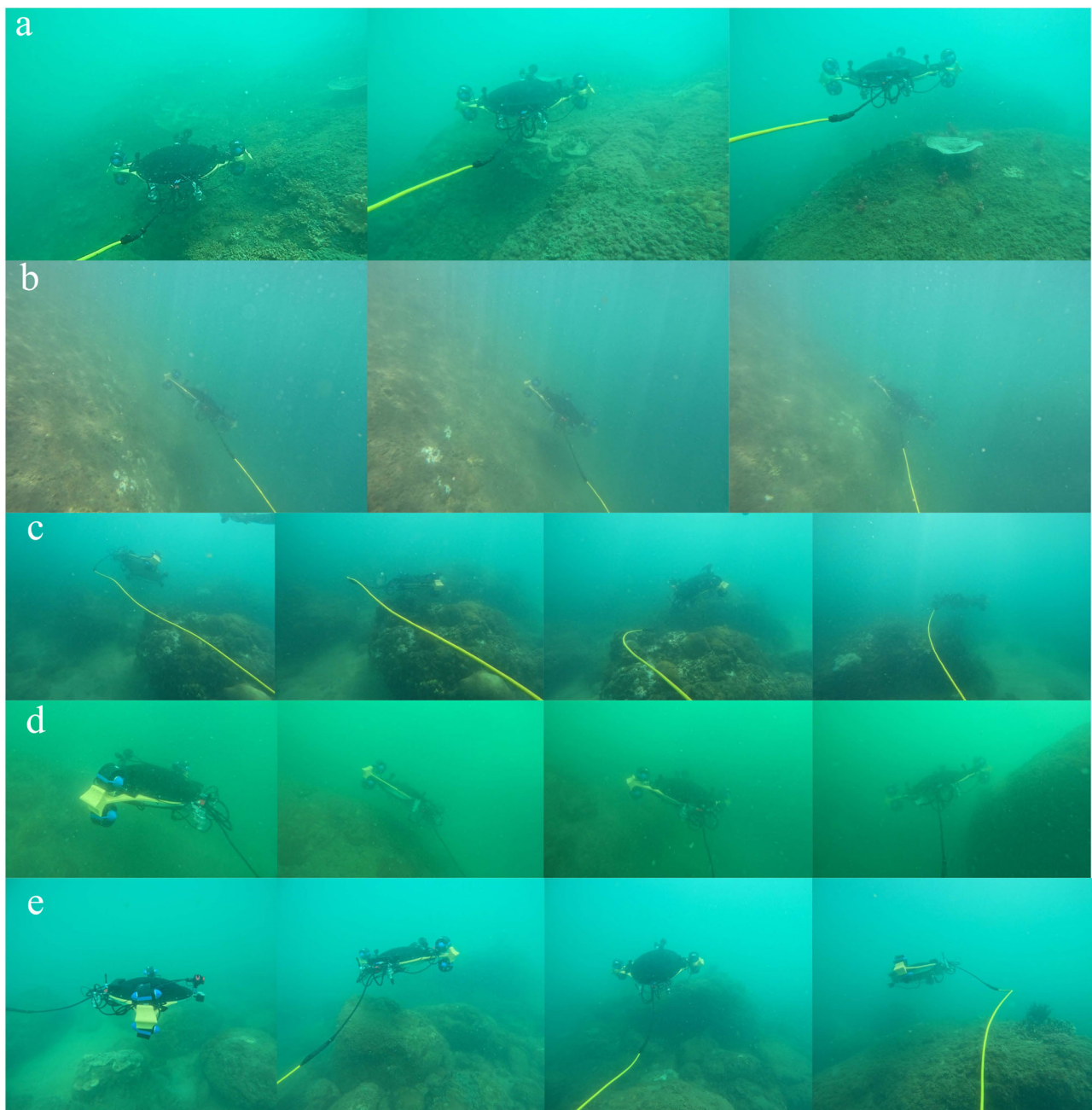
Fig. 8 | Field terrain tracking. a Ascending along a sloping terrain. b Using roll motion to closely approach a sloped terrain. c Executing continuous pitch maneuvers to traverse undulating terrain. d Performing roll maneuvers to evade obstacles ahead. e Field scanning motion.
