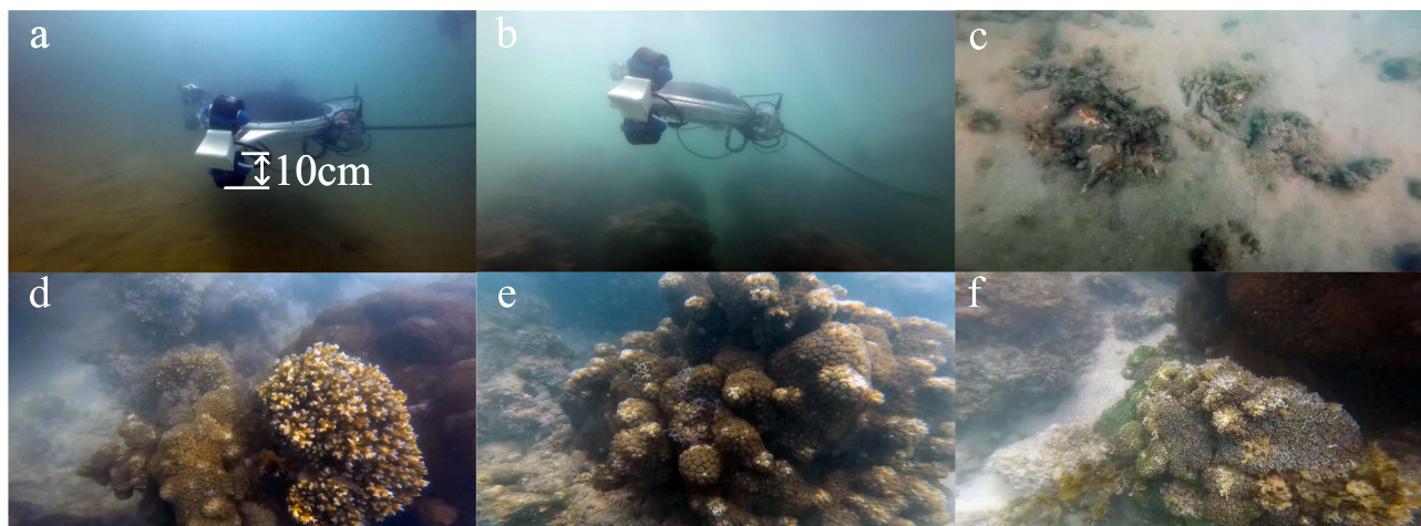
Fig. 1 | Field experiment. a Movement over sandy-gravel terrain, the diameter of the propeller fairing is labeled. b Upper coral reef movement. c Images of sandy-gravel terrain. d–f Images of coral reefs.
