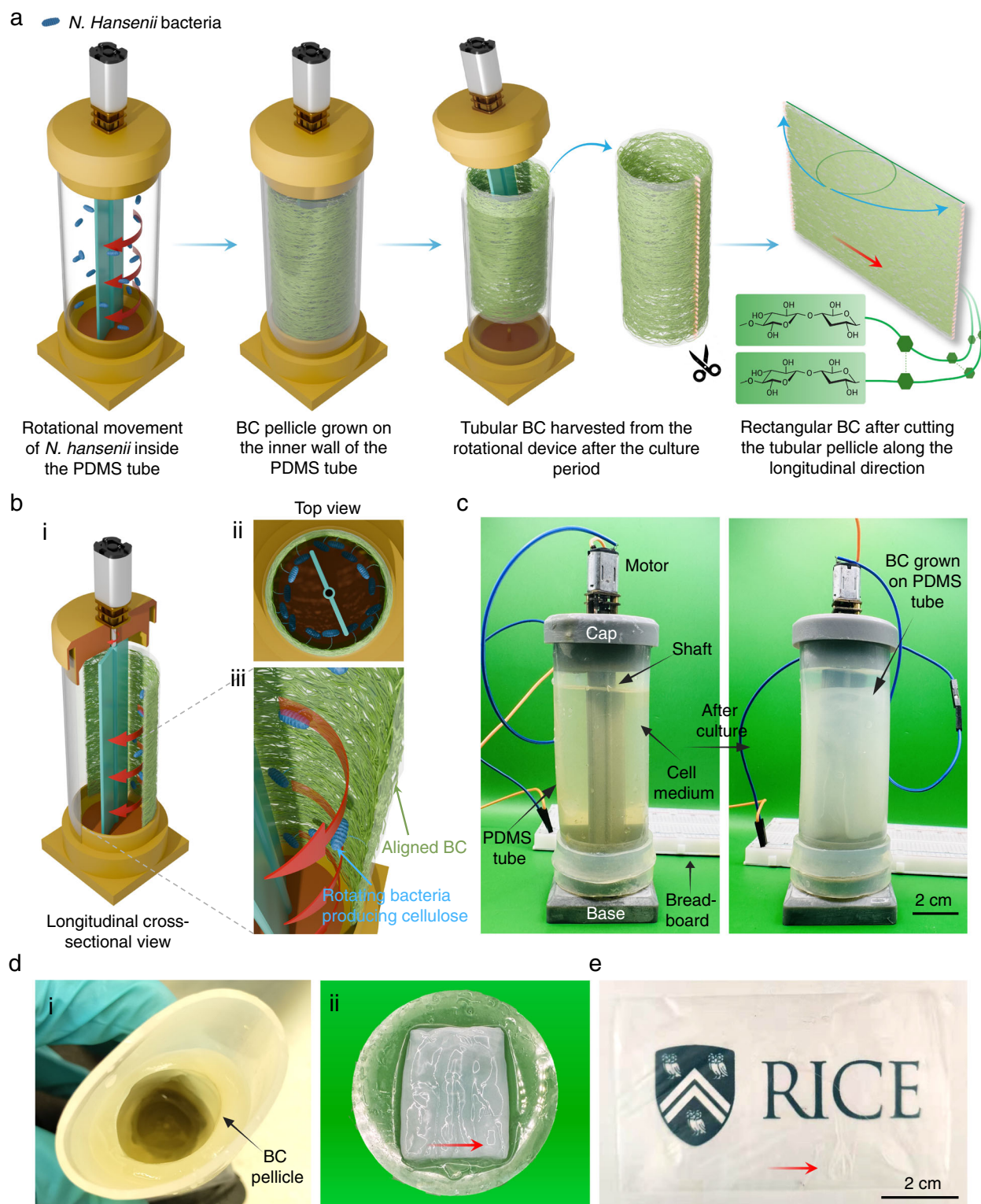
Fig. 1 | Fabrication of bacterial cellulose (BC) in rotation culture device.
