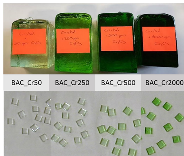
Fig. 1 | Images of the studied glasses with different amounts of chromium oxide. As-cast glass ingots are on the top of the image (5 cm wide and thick each) and polished monoliths are at the bottom, each measuring 5 × 5 × 2 mm.
