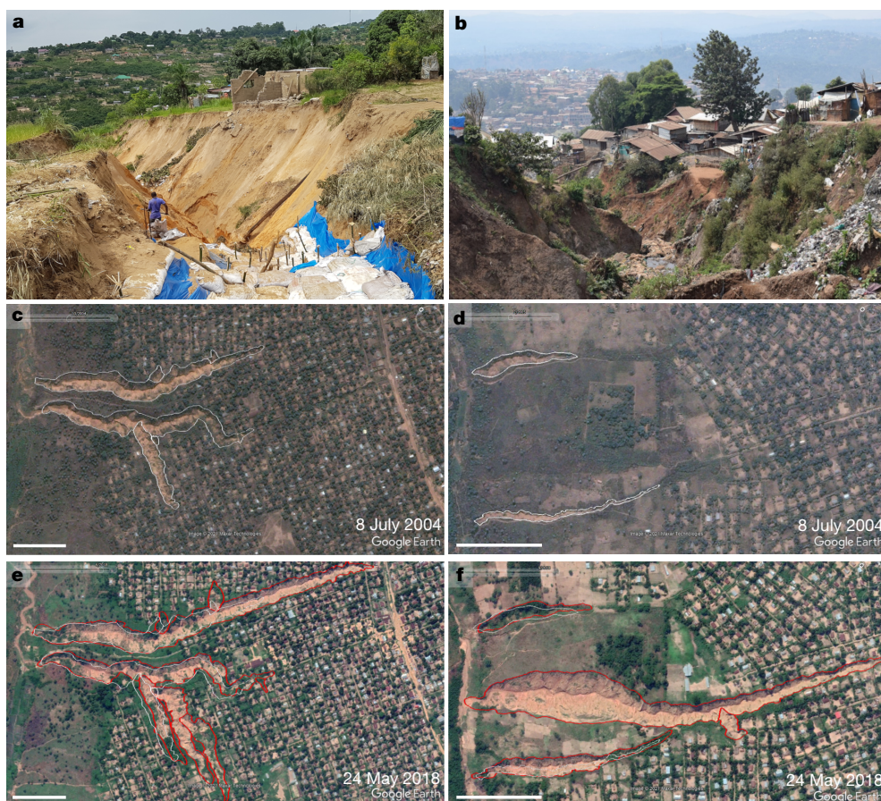
Fig. 1 | Examples of large UGs and the destruction they cause in the DRC. a , Tchad gully (Kinshasa, 26 November 2019). b , Funu gully (Bukavu, 8 July 2021). c, d , Google Earth imagery of UGs in Kikwit (8 July 2004). Gully extents
