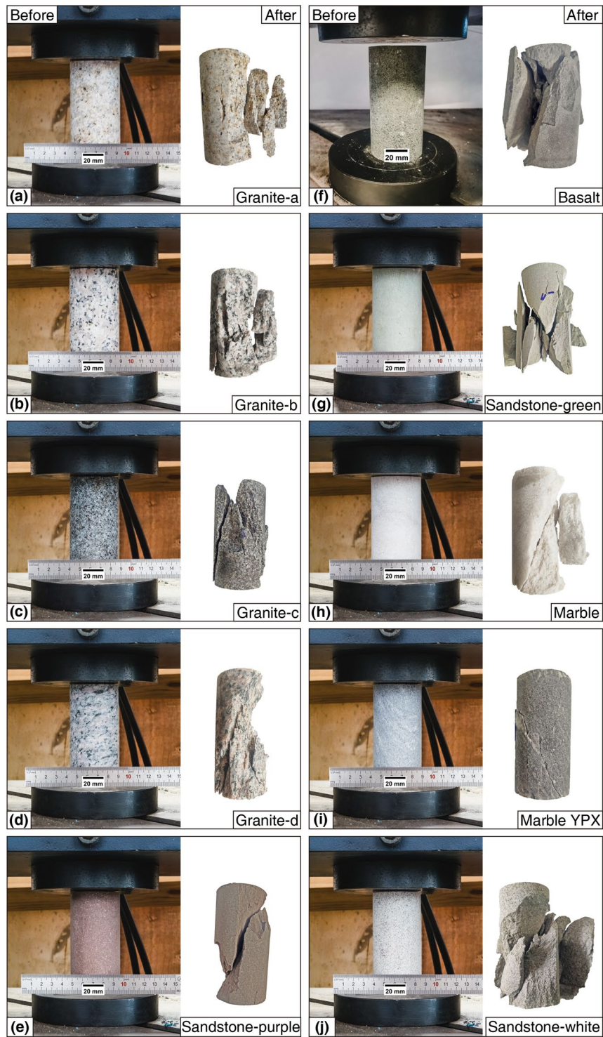
Fig. 7 The pictures of rock samples before and after the UCS test. (a) The images of Granite-a before and after UCS test, (b) The images of Granite-b before and after UCS test, (c) The images of Granite-c before and after UCS test, (d) The images of Granite-d before and after UCS test, (e) The images of Sandstone-purple before and after UCS test, (f) The images of Basalt before and after UCS test, (g) The images of Sandstone-green before and after UCS test, (h) The images of Marble before and after UCS test, (i) The images of Marble YPX before and after UCS test, (j) The images of Sandstone-white before and after UCS test.
