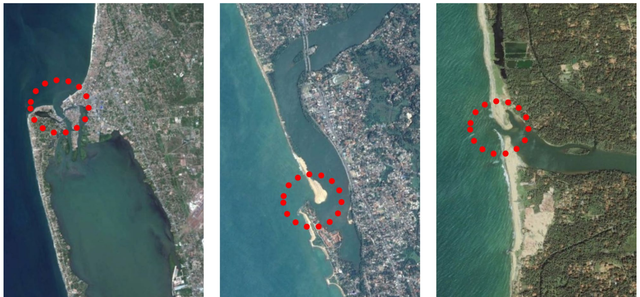
Figure 3. Negombo lagoon – Permanently open, locationally stable inlet: Type 1 (left), Kalutara lagoon – Permanently open, alongshore migrating inlet: Type 2 (middle), Maha Oya river – Seasonally/ Intermittently open, locationally stable inlet: Type 3 (right). The red dotted circles indicate inlet location (Reproduced from Duong et al. 24 , all rights reserved).
