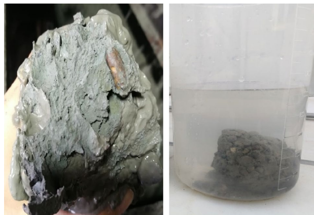
Figure 18. Mud cake sample was taken out from cutterhead.
