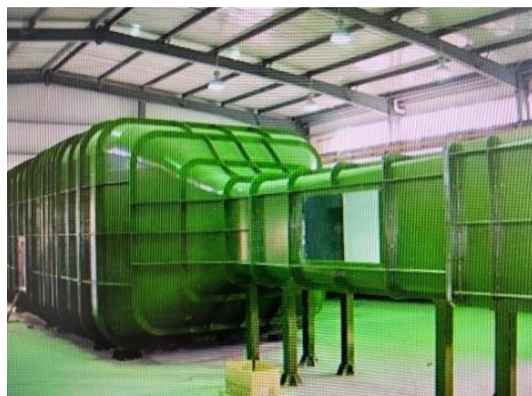
Figure 6. Low-speed backflow wind tunnel.
