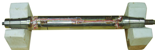
Figure 7. The schematic diagram of six-component for force-measuring balance.
