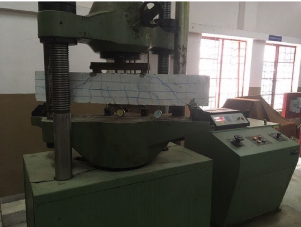
Figure 4. Test setup for RC beam.
