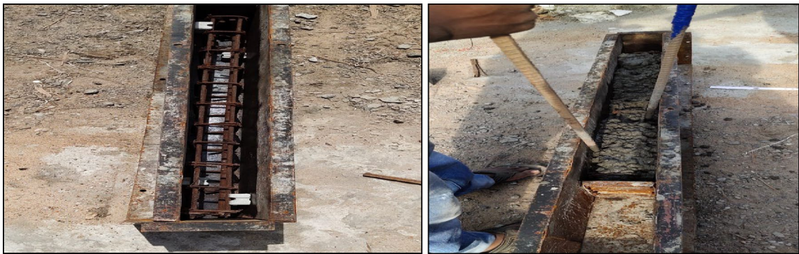
Figure 3. Casting of RCC beam.
