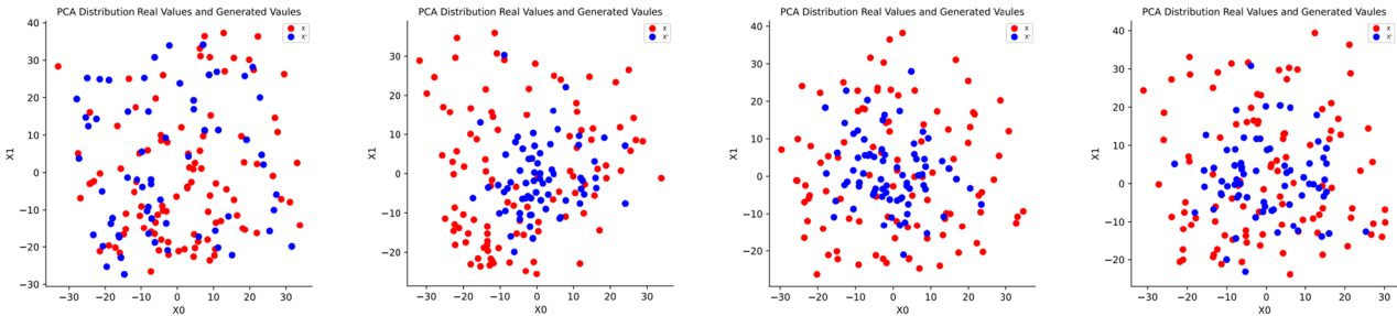
Figure 5. Two-dimensional principal component analysis of the Ship-D dataset reveals that the generated data using a standard DDPM maintained most of the dataset coverage. From left to right, the strategies corresponding are Base, EI, EI+HI, and EI+HI+AI.
