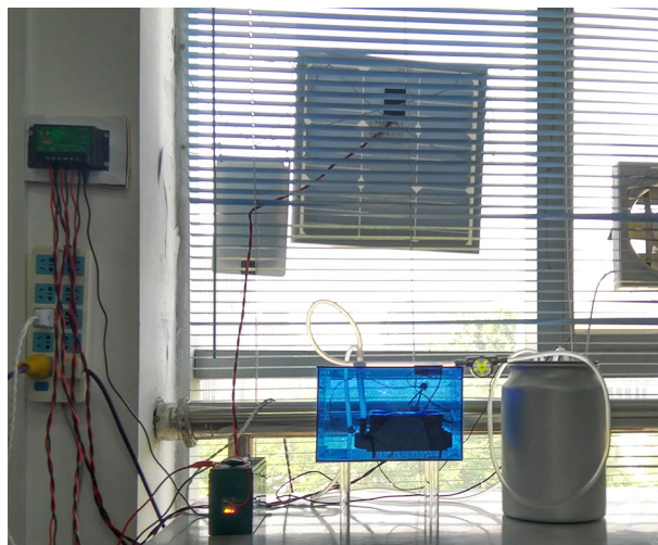
Figure 3. Photograph of the combined device including energy system and water recirculator. (Note: The water recirculator can be placed on the experimental table or fume cupboard using a long electric wire).
