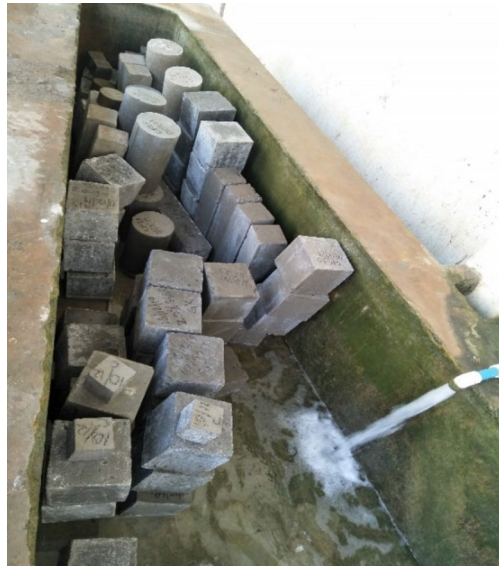
Figure 8. Curing of specimens.
