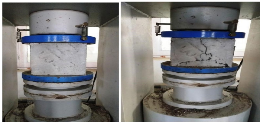
Figure 10. Compressive strength test.
