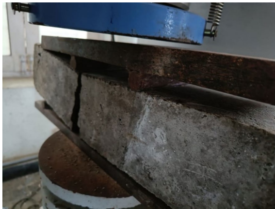
Figure 12. Split tensile test.
