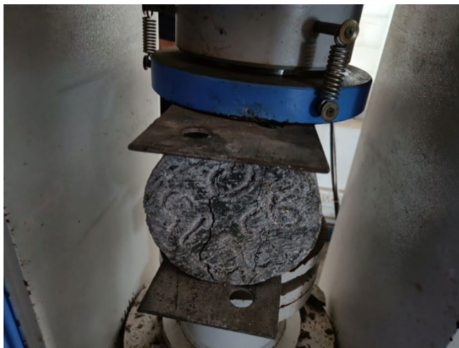
Figure 11. Split tensile strength test.
