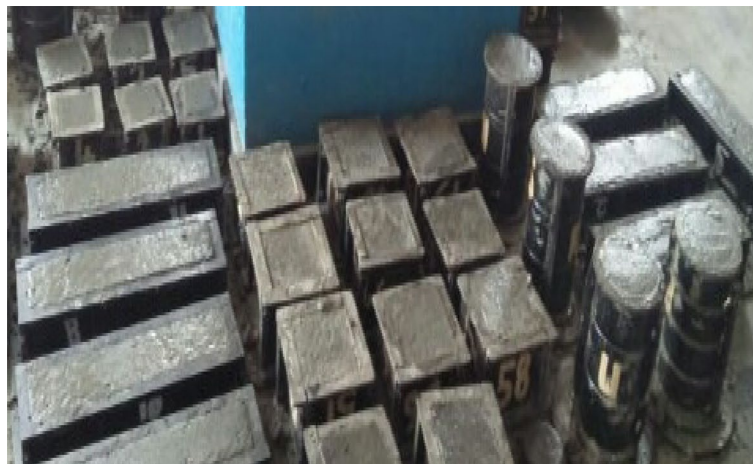
Figure 7. Casting of specimens.
