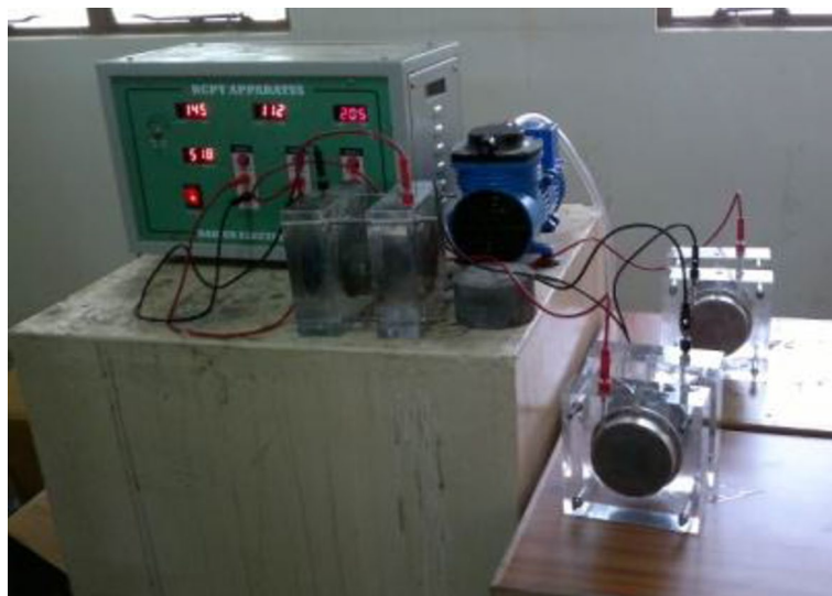
Figure 14. Chloride penetrability test.
