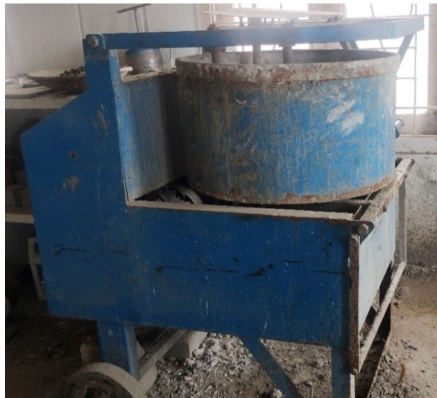
Figure 6. Mechanical drum mixer.
