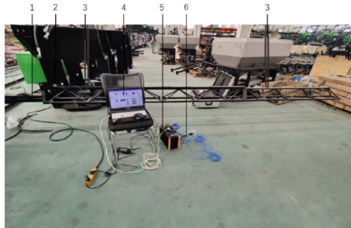
1. Spray boom truss 2. Accelerometer 3. Bungee cord 4. Computer 5. Dynamic Data Collector 6. Force hammer
