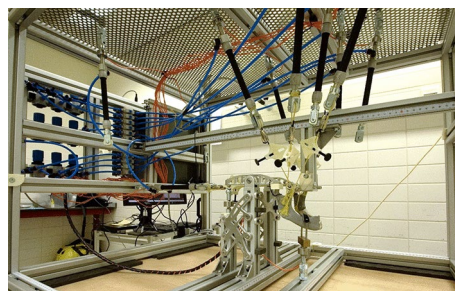
Fig. 4. Overview of the complete MANDYBILATOR apparatus with the mandible situated in the lower middle, the artificial muscles in the top middle and the electro-pneumatic controls on the left side.
