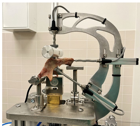
Fig. 3. A picture of the MUNACAPP apparatus ready for static uniaxial compressive testing of a cadaveric mandible.
