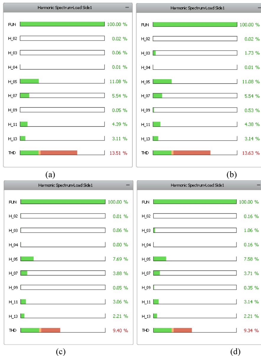
Fig. 16. Harmonic spectra of load current under a sudden load change—(a) before the load change under balanced PCC voltage condition, (b) before the load change under unbalanced PCC voltage condition, (c) after the load change under balanced PCC voltage condition, and (d) after the load change under unbalanced PCC voltage condition.
