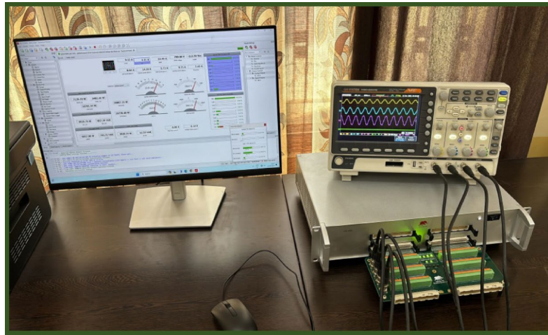
Fig. 3. Typhoon HIL 604 simulator used for real-time simulation of the PV-DSTATCOM system.
