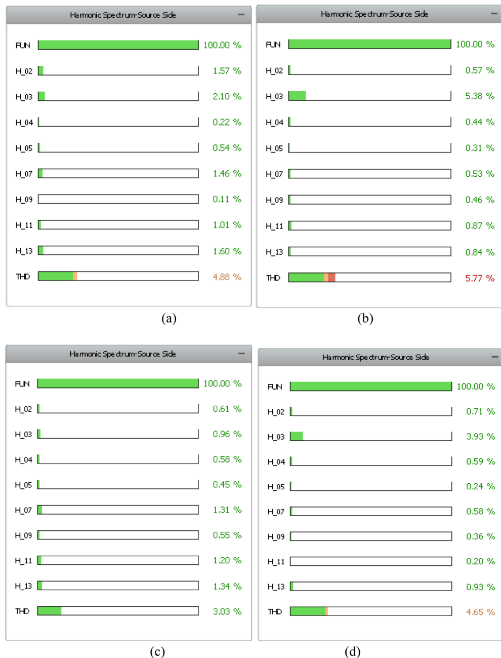
Fig. 20. Harmonic spectra of source/grid current under a sudden load change at an irradiance level of 700 W/m²—(a) before the load change under balanced PCC voltage condition with PV power injection at an irradiance level of 700 W/m², (b) before the load change under unbalanced PCC voltage condition with PV power injection at an irradiance level of 700 W/m², (c) after the load change under balanced PCC voltage condition with PV power injection at an irradiance level of 700 W/m², and (d) after the load change under unbalanced PCC voltage condition with PV power injection at an irradiance level of 700 W/m².
