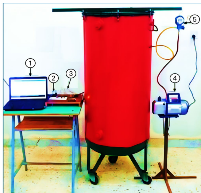
Fig. 1. Main components of the DAVD. Whereas (1) Laptop, (2) Arduino uno board, (3) Control unit, (4) Vacuum pump, and (5) Vacuum gauge.
