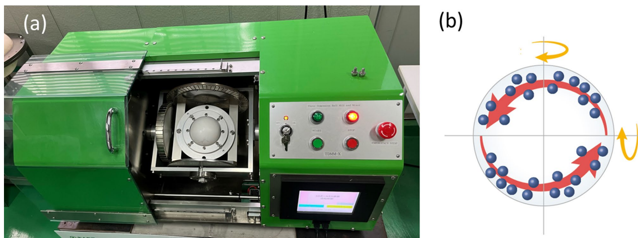
Fig. 1. (a) Three-dimensionally driven ball mill machine. Crushed solids are fed into the spherical container in the centre of the machine. (b) Image of driving a ball mill vessel.
