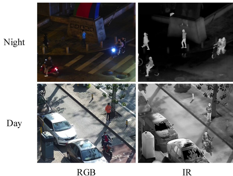
Fig. 1. The first column is a RGB image and the second column is an IR image. The first row captures images taken at night, where the infrared image distinctly highlights the positions of pedestrians. In contrast, the second row showcases daytime images, in which the visible light photograph distinctly highlights the background details.
