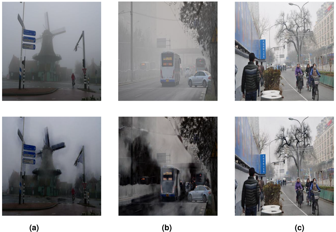
Fig. 9. The images processed by the proposed DSNet model are presented, where the first row shows the original foggy images, and the second row displays the corresponding dehazed results.
