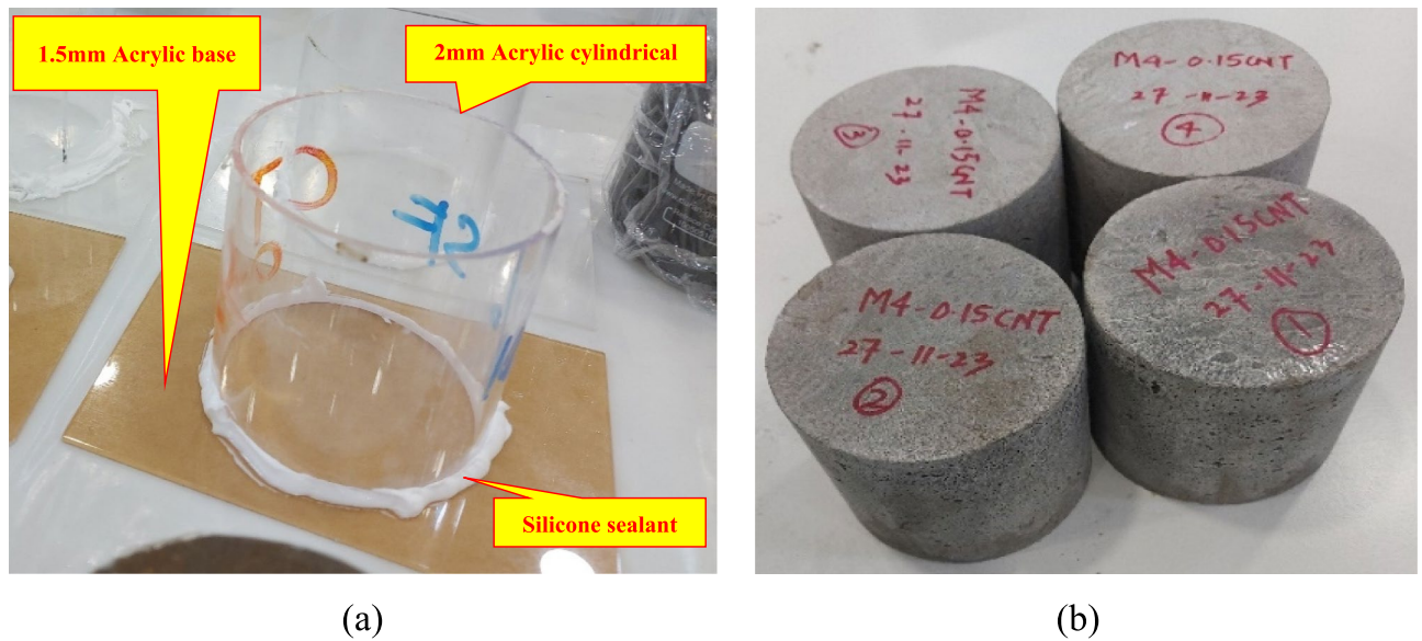
Fig. 3. Preparation of cylindrical specimens: (a) custom-made acrylic mold sealed with silicon sealant at the bottom to check the leakage of water and cement and (b) cylindrical specimens with 96 mm diameter and 80 mm depth.
