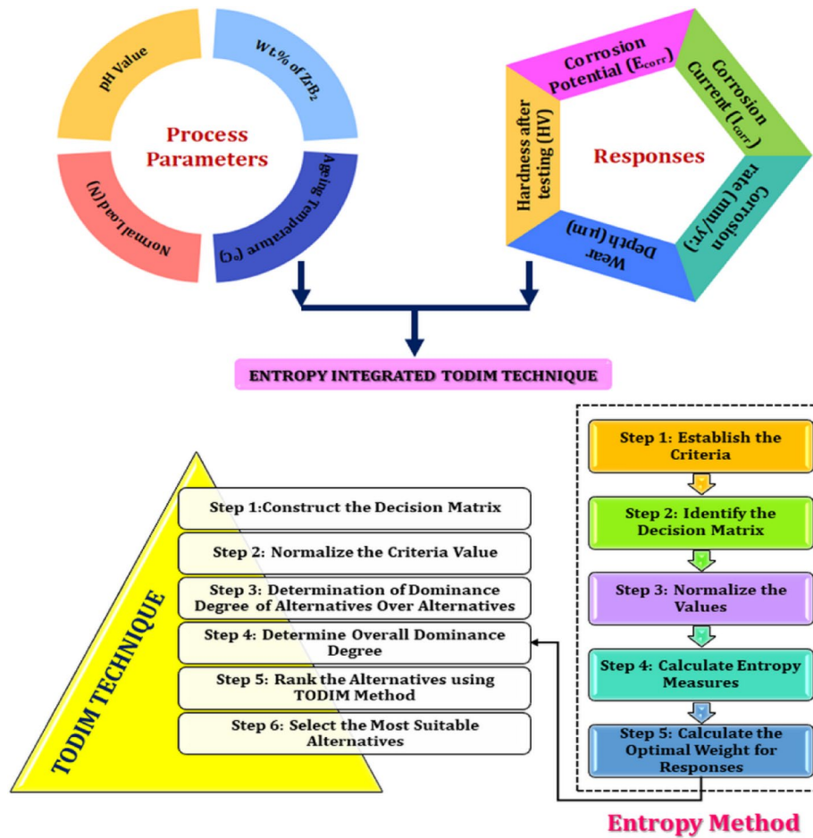
Fig. 5. Flow diagram of the proposed methodology.
