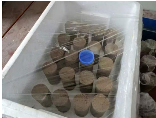
Fig. 4. The process of triaxial samples preparation.
