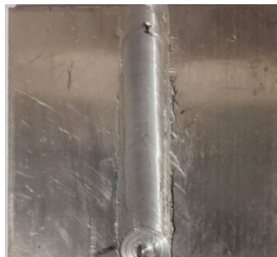
Fig. 4. Macroscopic image of the friction weld sample.
