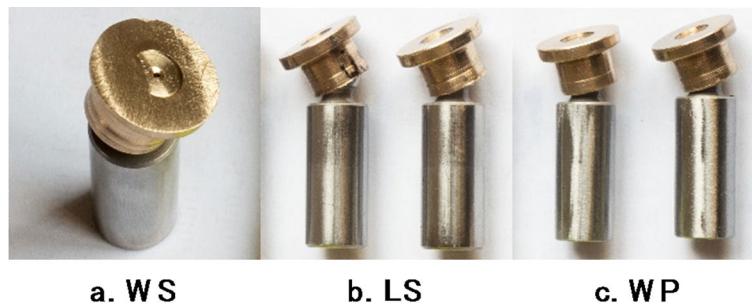
Fig. 7. Photographs of faulty parts for hydraulic pump tests.
