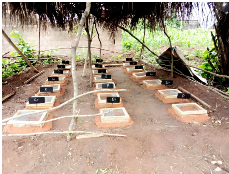
Fig. 2. Design layout of the underground clay-composite storage chambers.
