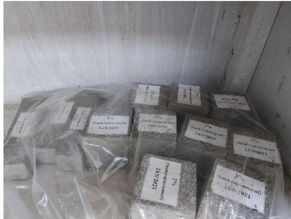
Fig. 5. Specimens during the treatment process.
