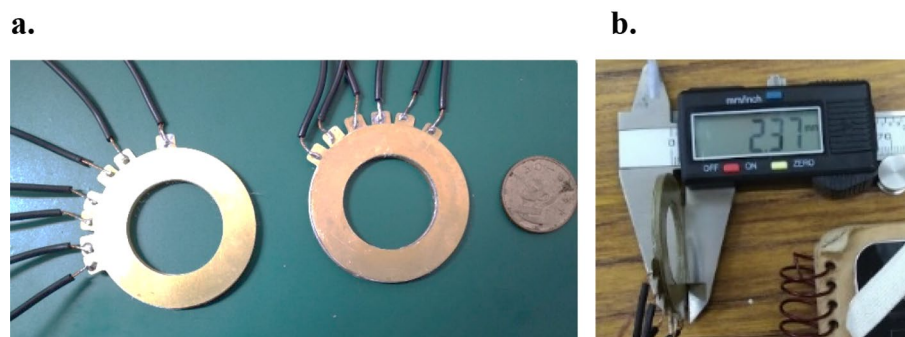
Fig. 11. (a) Sample size and (b) the thickness measurement using a vernier caliper.
