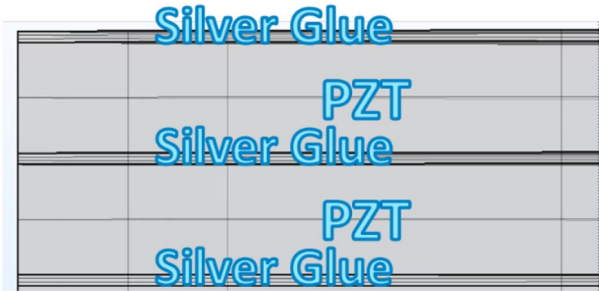
Fig. 1. Mesh side cutting diagram of piezoelectric material.
