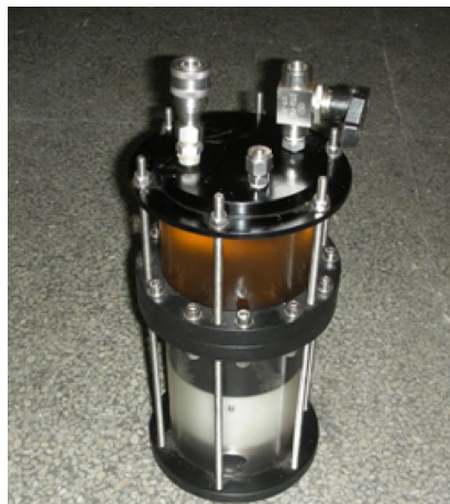
Fig. 9. Schematic diagram of pressure-compensating component.
