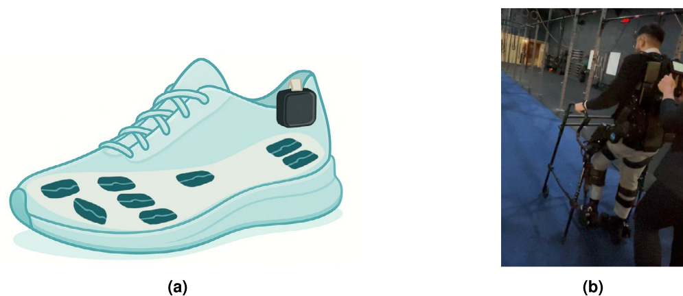
Fig. 1. Experimental setup and equipment configuration. (a) Configuration of the smart insole system used in the experiments, showing its placement inside the user's shoe. Each insole was equipped with 8 pressure sensors and an Electronic Control Unit (ECU) containing Inertial Measurement Unit (IMU) sensors. The illustration was created by the authors using Photopea version 5.6. (b) Image of co-author Luigi D'Arco, who provided consent for the use of this photograph, wearing the smart insoles and an exoskeleton during data collection. The setup also includes a walking aid and support from a physiotherapist.
