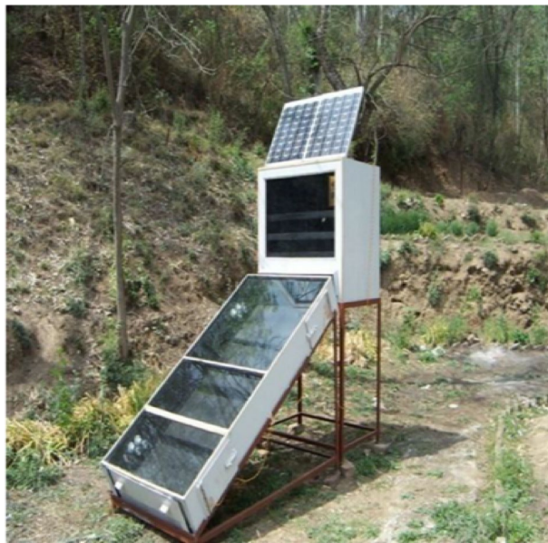
Fig. 9. Constructed model of the indirect solar dryer for practical use 27 .
