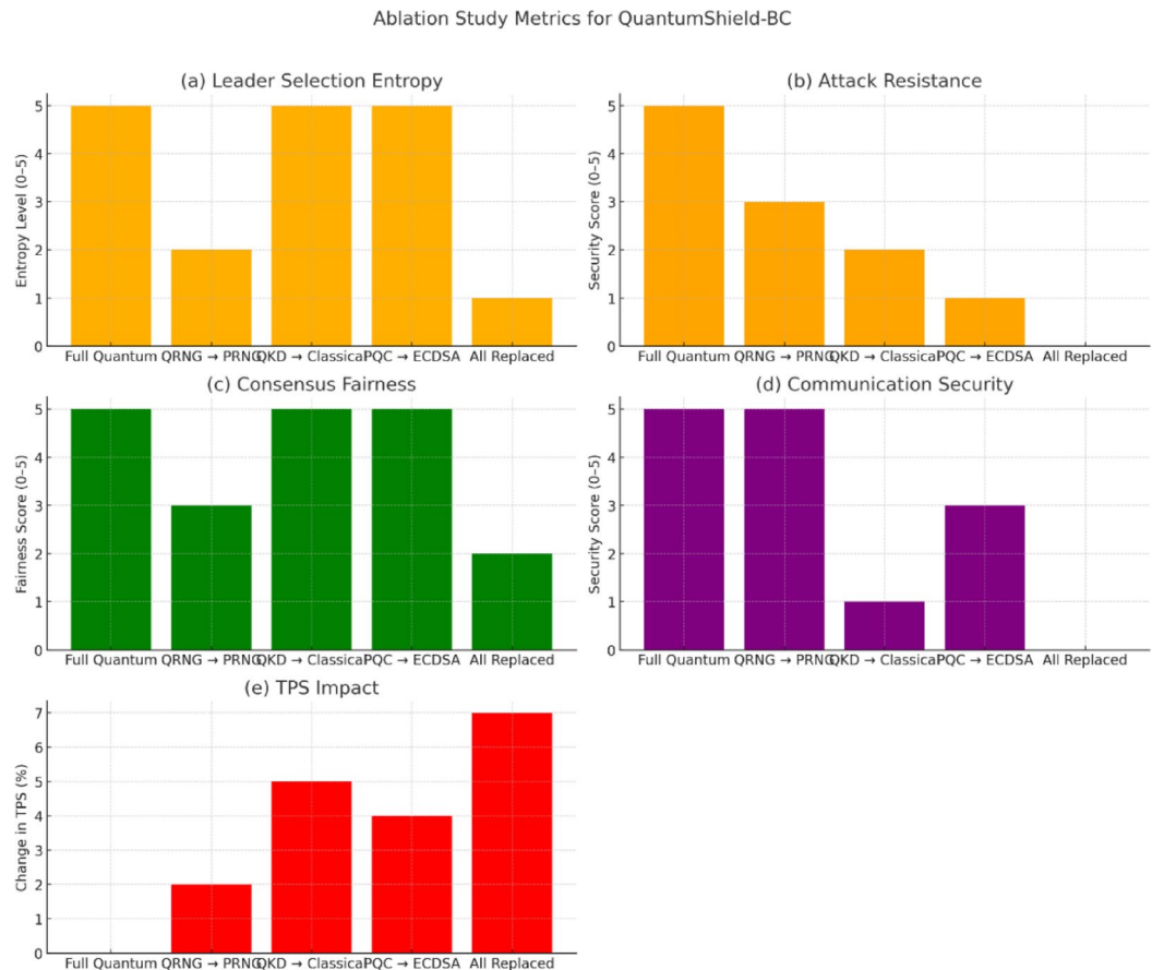
Fig. 6. Ablation study results showing the impact of disabling QRNG, QKD, and PQC on entropy, security, fairness, communication integrity, and transaction throughput in QuantumShield-BC.
