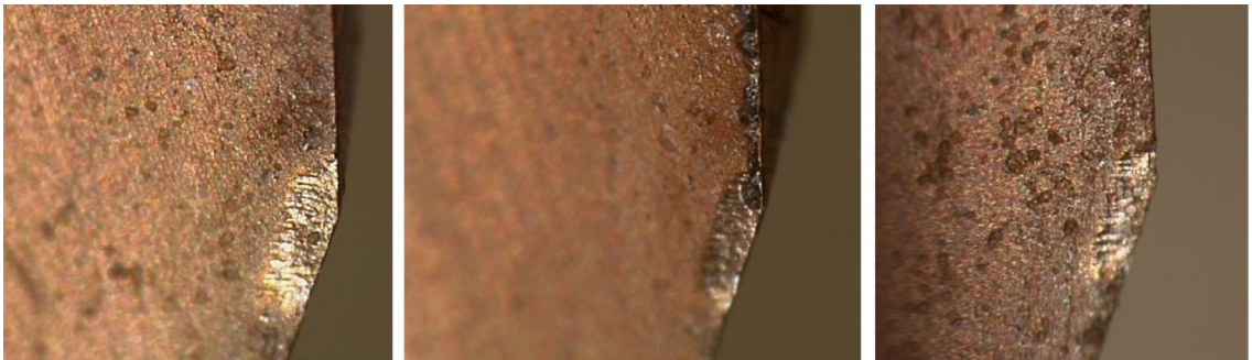
Fig. 9. An enlarged image of the worn front cutting surface.
