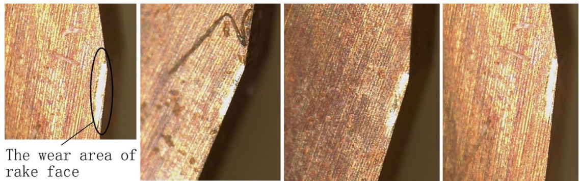
Fig. 13. Wear appearance of rake face.
