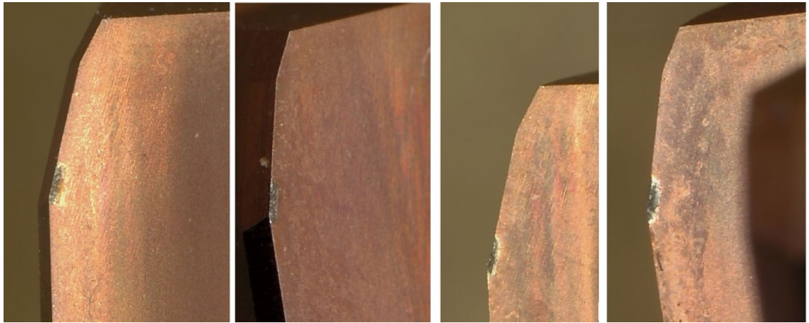
Fig. 8. Failure diagram of cutting edge wear.
