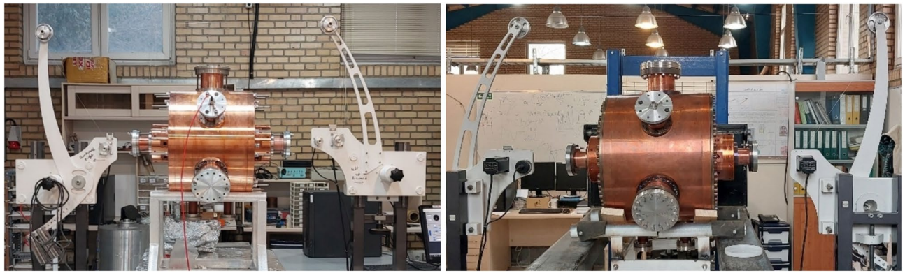
Fig. 25. The HHC parts screwed together for low-power RF measurements (left) and after the final brazing (right). The bead pull measurement setup is also illustrated in the figures.
