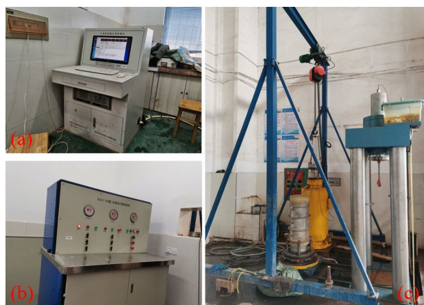
Fig. 5. The DJSZ-150 large-scale dynamic and static triaxial testing machine: (a) computer control system, (b) pressure control system, (c) loading system.
