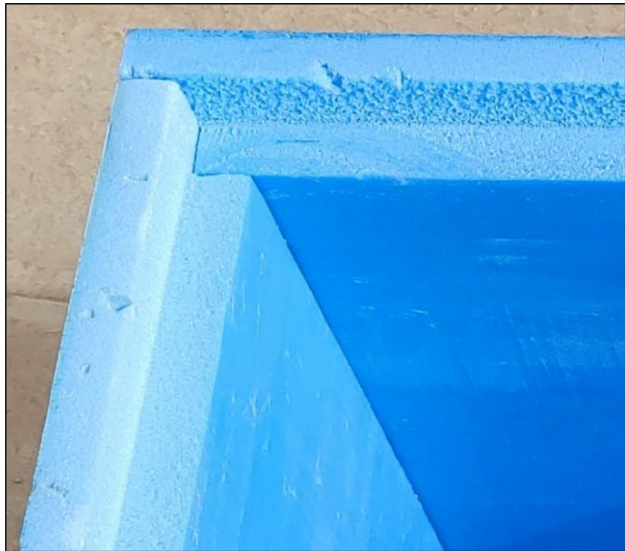
Fig. 6. Half-lap Joint connection of the box’s sides.
