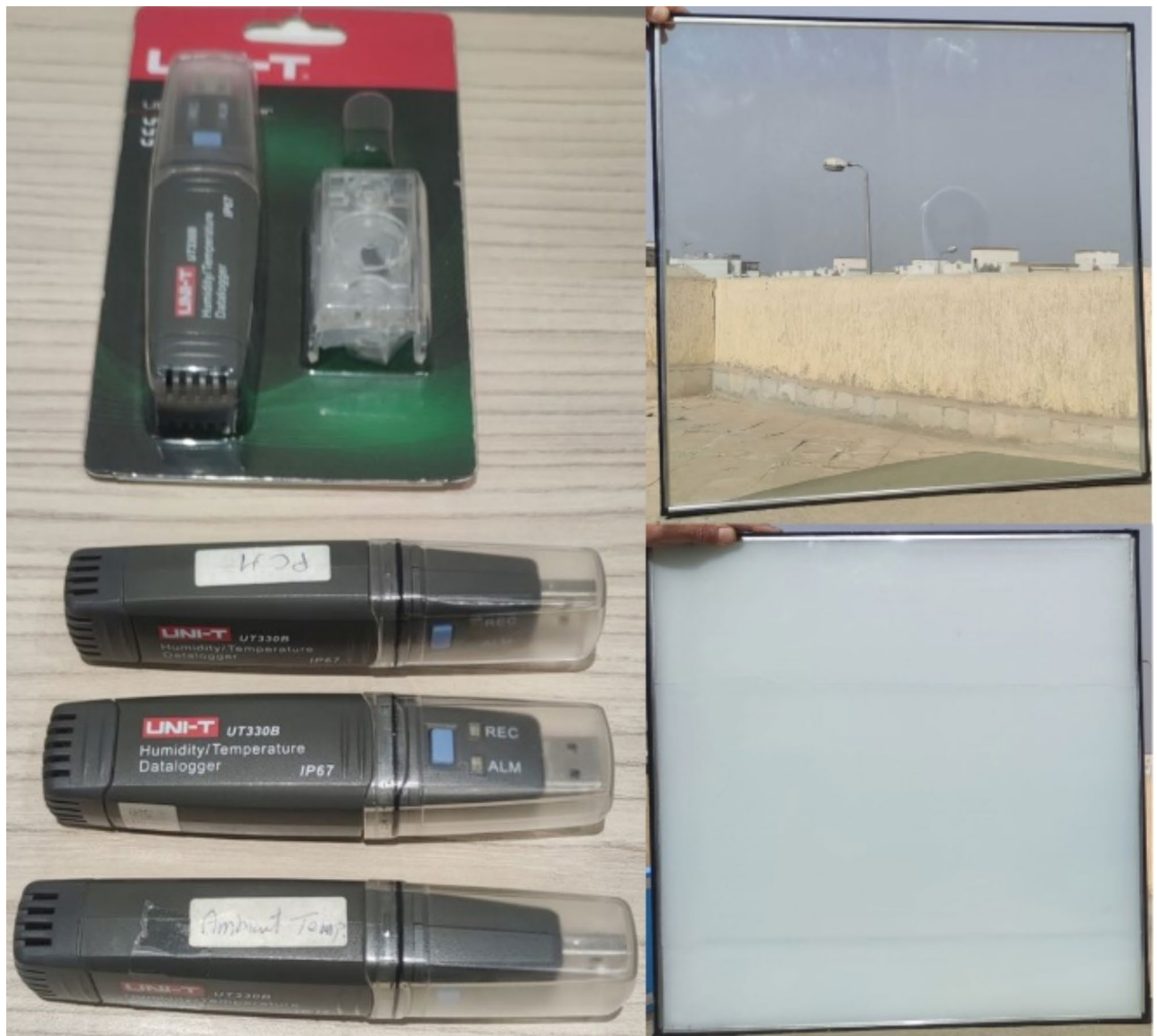
Fig. 5. (Left) set of dataloggers used through the experiment. (Up right) DGU with air gap. (Down right) DGU with PCM in solid state.
