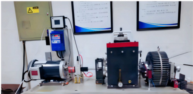
Fig. 12. Fault diagnosis test bench for gearbox at Southeast University.
