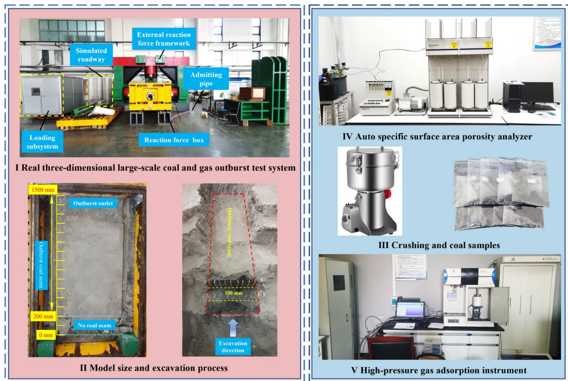
Fig. 1. Determination of pore structure and desorption characteristics of coal and gas outburst coal samples.
