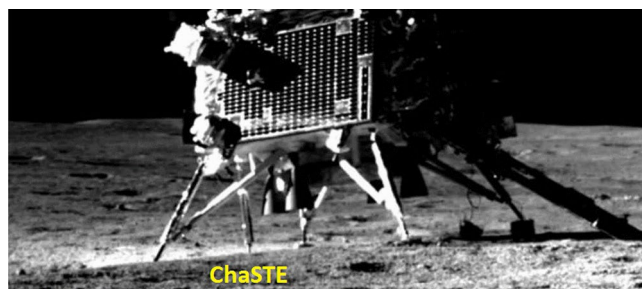
Fig. 6. Image of Chandrayaan 3 Vikram lander at Shiv Shakti landing site taken by Pragyan rover navigation camera. ChaSTE is seen in the penetrated configuration.
