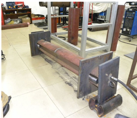
Fig. 11. ECP specimen before pressurization.
