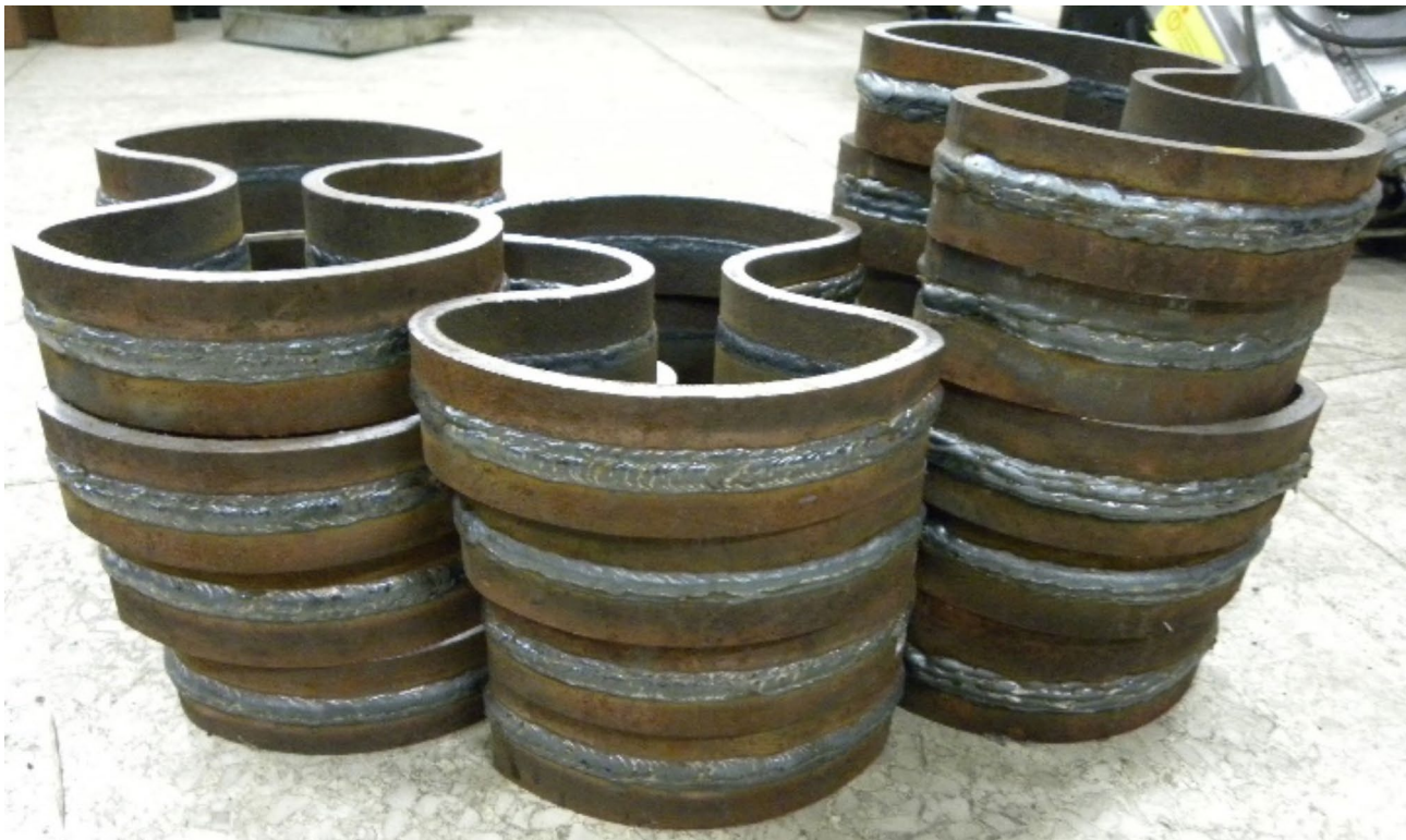
Fig. 10. Welding test specimens of ECPs.
