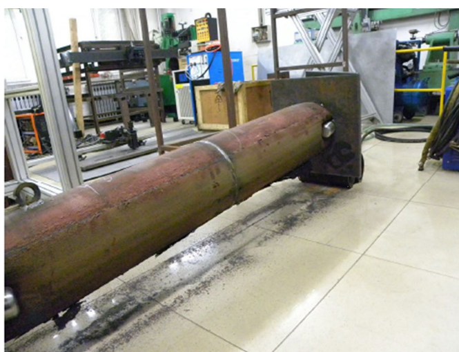
Fig. 12. ECP specimen pressurized to 26 MPa.
