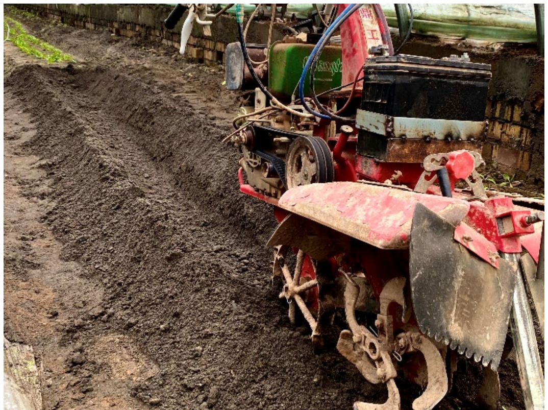
Fig. 14. Trenching test conducted under river sand substrate.
