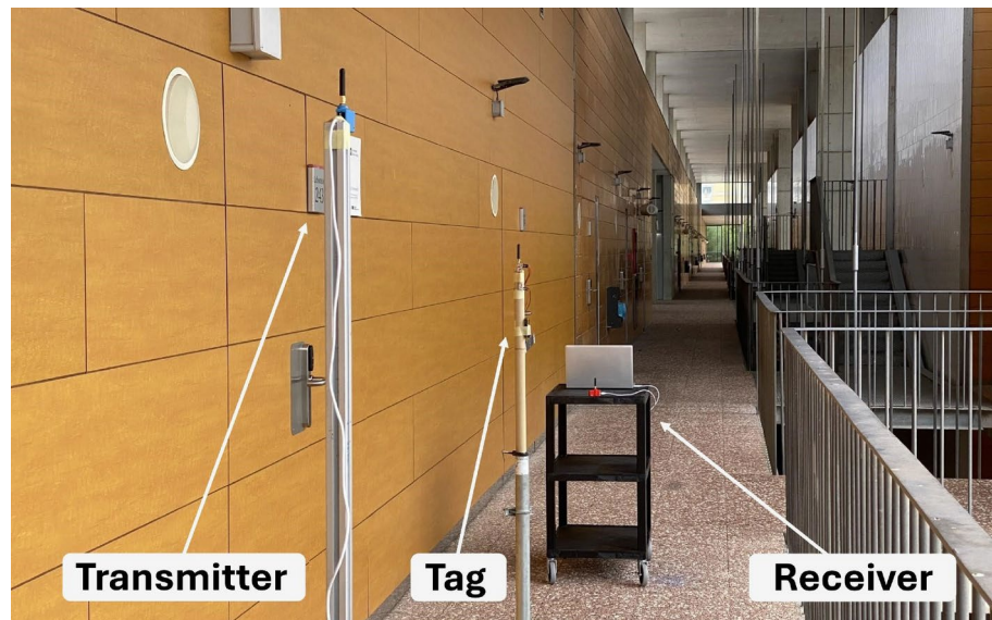
Fig. 21. Photograph of the measurement setup and environment used to validate the coverage enhancement of the reflection amplifier.
