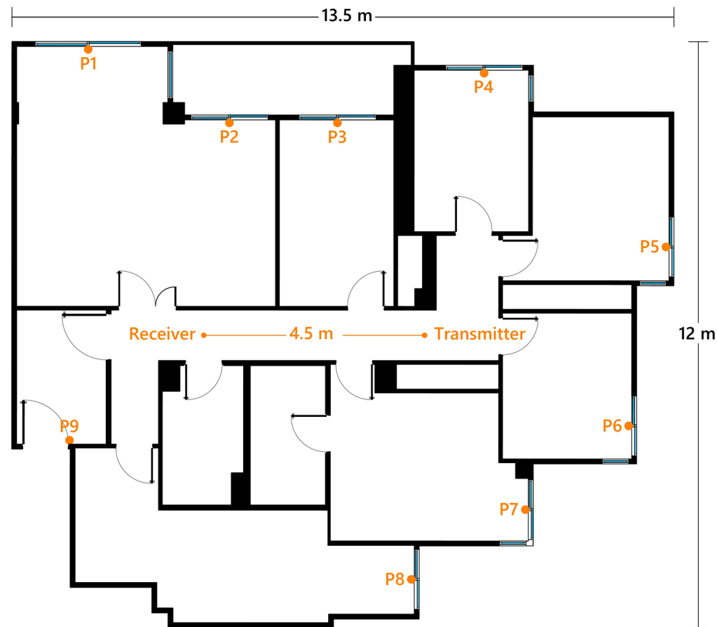
Fig. 19. Layout of the apartment where measurements are conducted, showing the positions of the transceivers and the assessment points for the wireless sensor (P1–P9).
